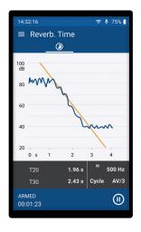
The standard reverberation time measurement determines T20 or T30 in octave bands from 63 Hz - 8 kHz. The values of a measured position or of an entire room are averaged on the XL3. The optional Room Acoustics Package extends the Acoustic Analyzer to 1/3 octave band resolution, T15 or EDT. Use either an impulse source or an interrupted pink noise as the test signal.
