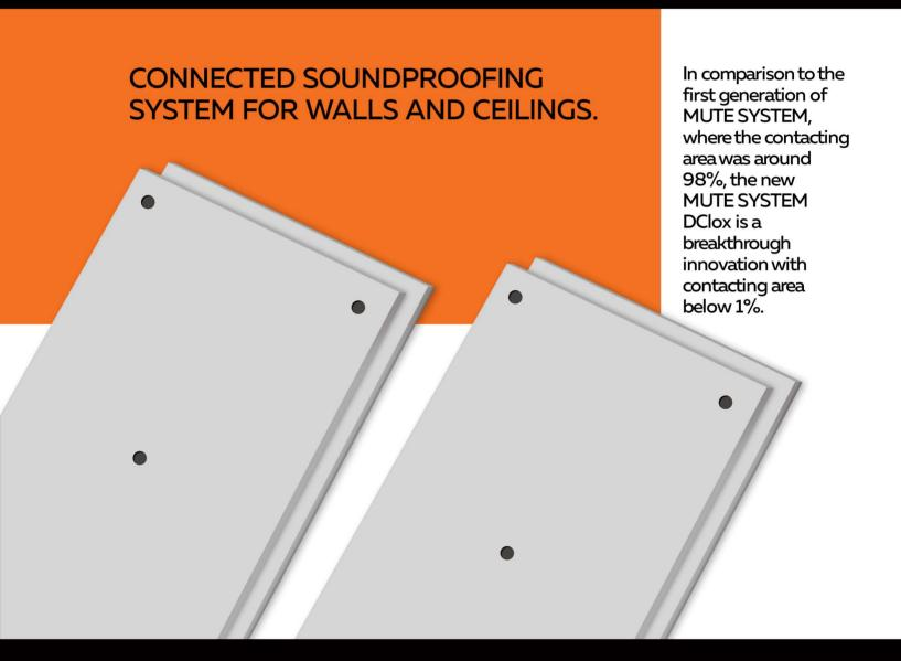
The system is easy to mount via specially designed anti-vibration DClox element, patented in the EU. DClox point connection ensures less than 1% contact area between the soundproofing panels and the existing partition thus ensuring minimal sound transmission.
